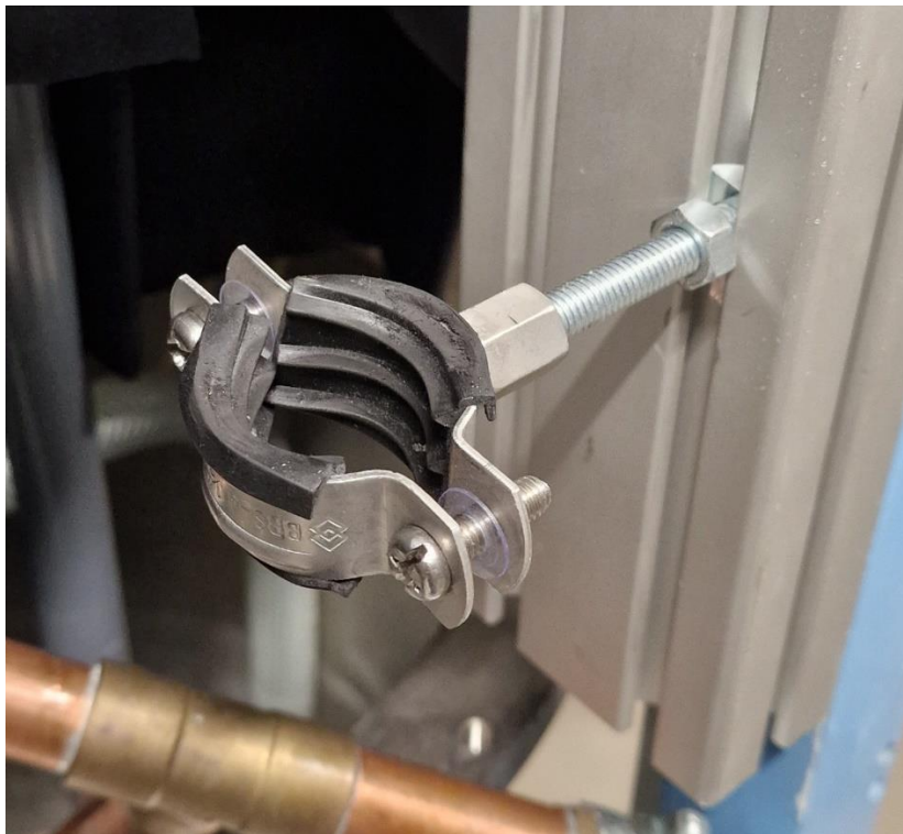
Figure 64. Bottom bracket of the flotation column, wear on the contact surfaces can be observed.
