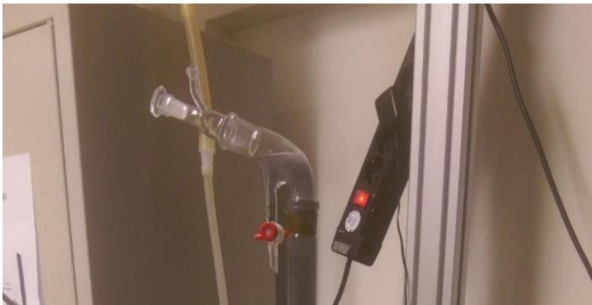
Figure 18. The Hallimond tube used in previous experiments.
