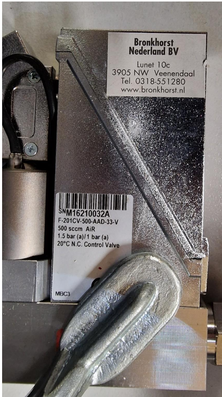
Figure 65. Image of the used mass flow controller.
