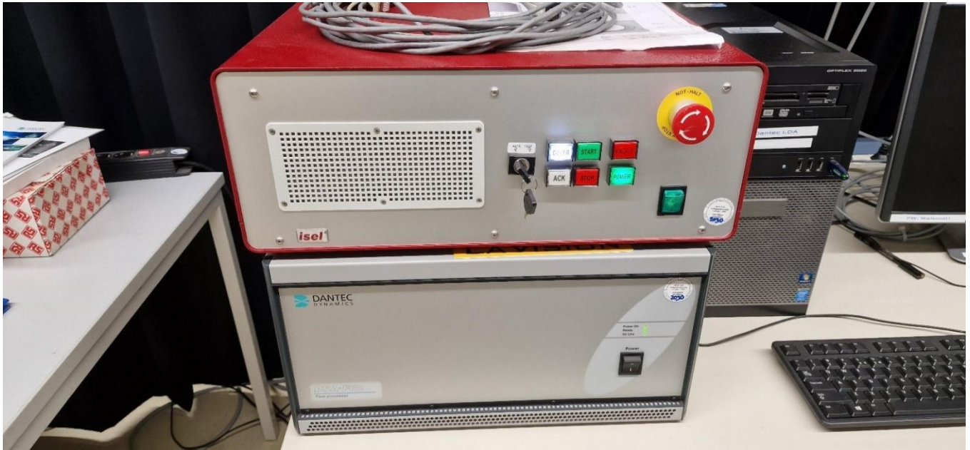
Figure 15. Top: Control unit of the traverse. Bottom: the Burst Spectrum Analyzer.
