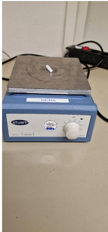
Figure 66. Image of the magnetic mixer used in two-phase flows.
