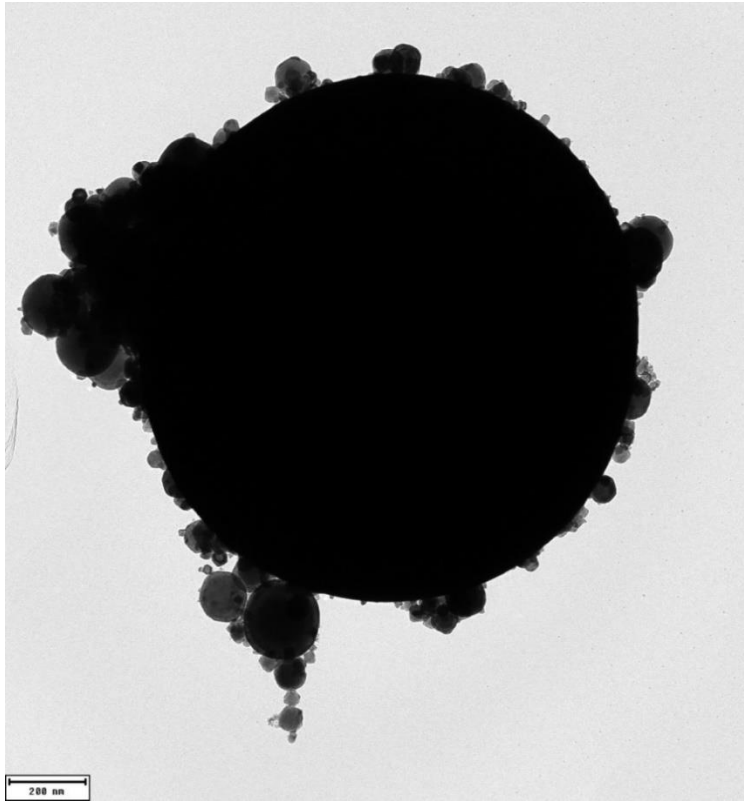
Figure 21. Example of a cluster in the sub 100 nm powder under TEM with a size scale of 200 nm.
