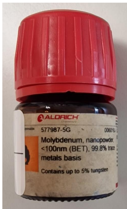
Figure 58. Image of the used sub 100 nm molybdenum powder.
