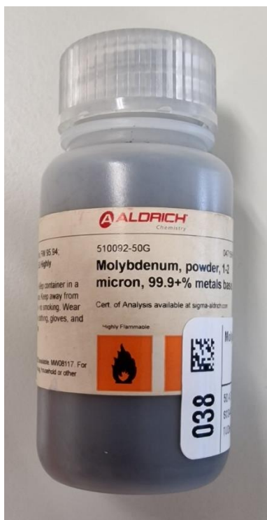
Figure 57. Image of the used 1-2 micron molybdenum powder.
