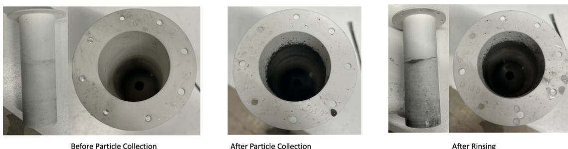
*Figure A1: 500 nm nickel particles before particle collection, after particle collection, and after rinsing.*
